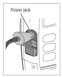
**CAUTION:** Failure to push the connector all the way forward may result in an intermittent connection, and the connector may dislodge, causing a loss of power.
